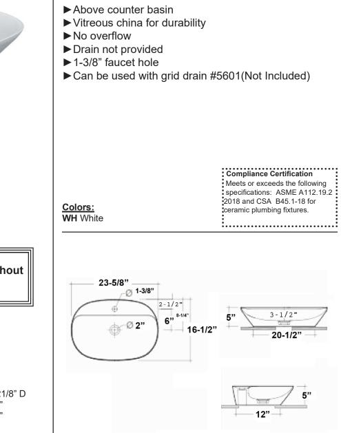
Dimensions of fixture are nominal and may vary within the range of tolerances established by AMSE Standard A112.19.2.2013 Dimensions and specifications subject to change without notice.
